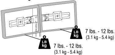
Total weight of monitors when mounted needs to be 14 lbs - 24 lbs (6.2 kg - 10.8 kg)
